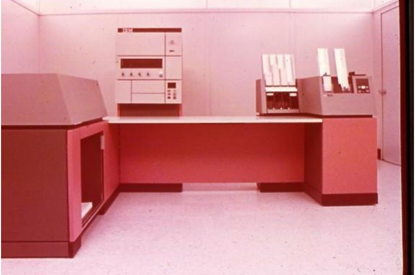
Figure 7-5 IBM System/3 Model 10 with MFCU (Right) and Printer (Left)
