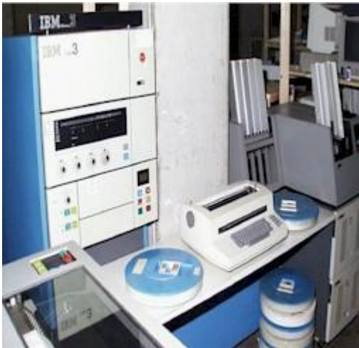
IBM System/3 Disk System, card unit and printer circa 1971--One-Third the Size, 20 Percent More Data
