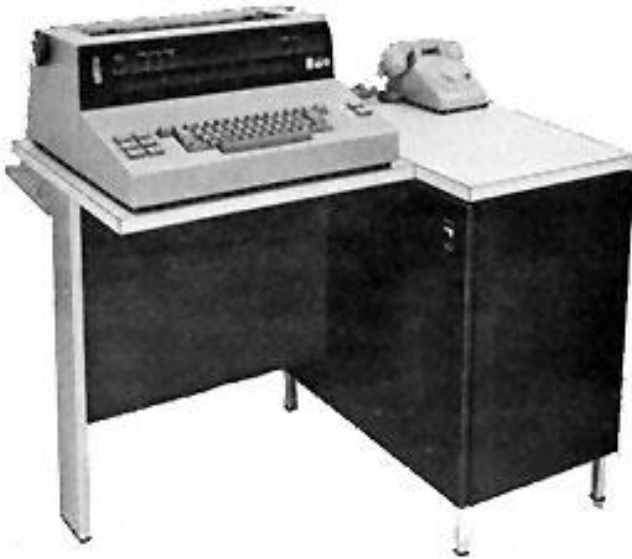
Figure 41-1 IBM 1050 Data Communications System
