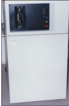
Figure 1-4 IBM System/34 Multi-Station Computer
