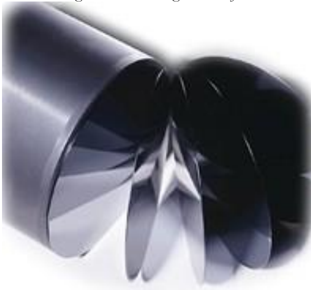
Figure 3-2 Sliced Ingot & Wafers
