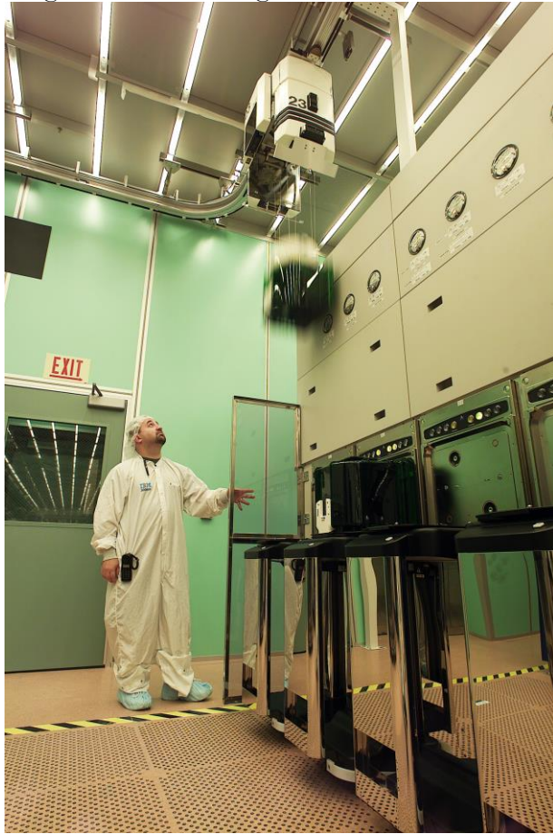
Figure 3-6 FOUP Being Snatched Back into R2D2
