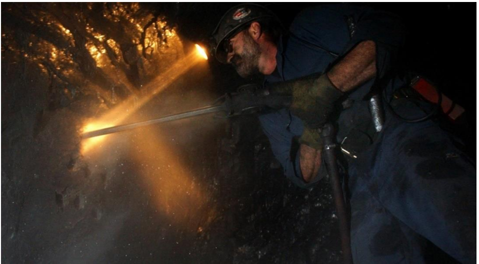
Miner Pete Wenrich drills into wall rock to place dynamite at the RS&W Anthracite Coal Mine in Pottsville in 2003. (Carolyn Kaster/Associated Press)
